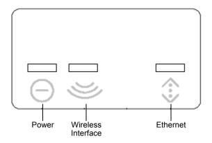
Figure 2-3 LED Indicators on the Top Panel
